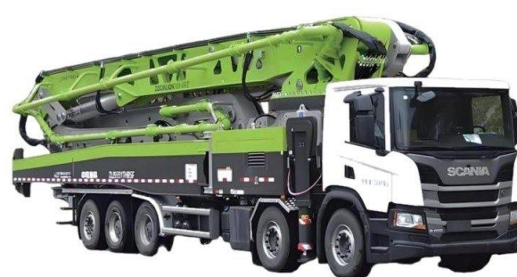
Concrete pump truck · ZOOMLION
